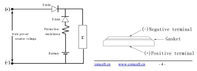
Back-current Prevention D iode and Protection Resistor U sed
